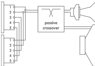
**Fig. 2: Connector wiring**
