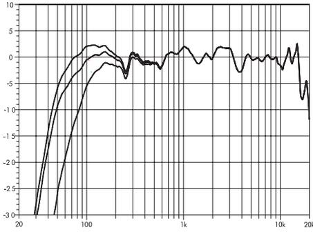
**Fig. 7: E9 frequency response standard, BX and CUT switch settings**
