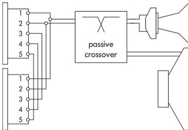
**Fig. 2: Connector wiring**
