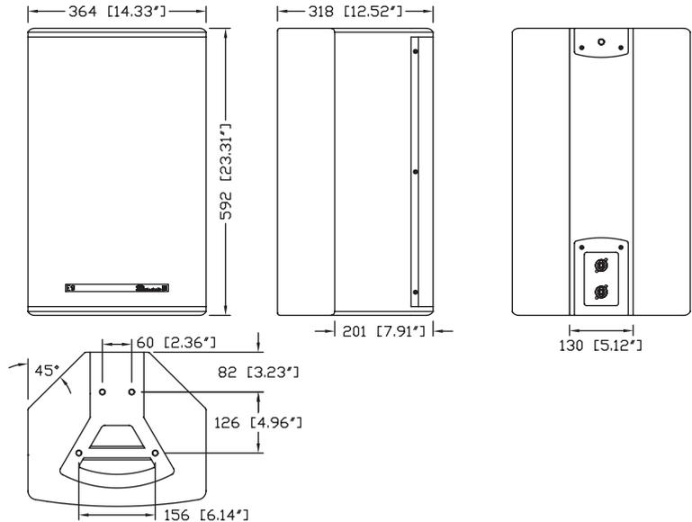
**Fig. 8: E9 cabinet dimensions in mm [inch]**
