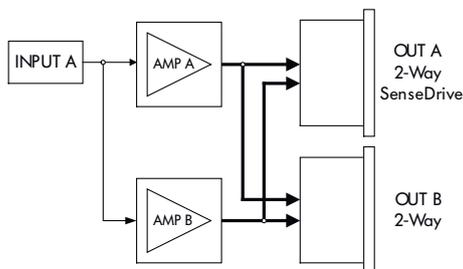
**D12 Input/Output routing 2-Way Active mode**
